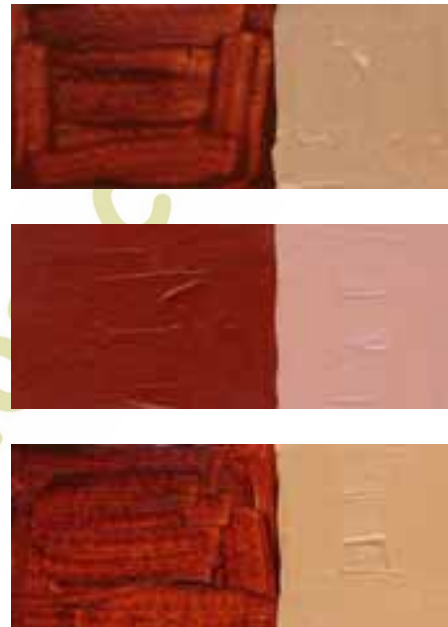
Figure 6: Natural Burnt Sienna (PBr7), Venetian Red (PR101) and Transparent Red Iron Oxide (PR101).
